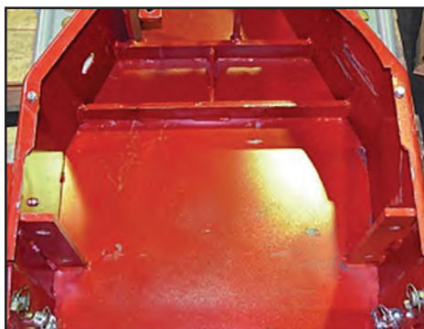
12 - Use a hammer again to "pean over" the box brackets to hold the clutch pads in place.
