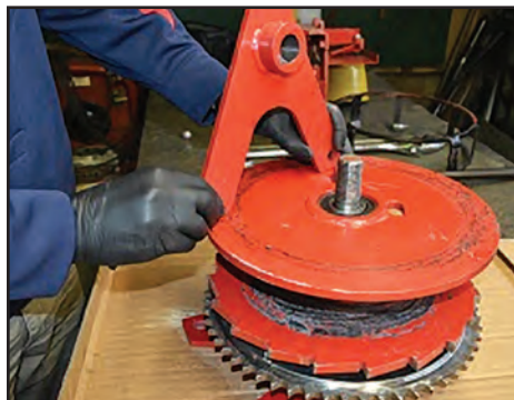
6 - Take off the connecting bracket from the drum unit.
