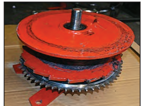
7 - The drum unit is now ready to separate from the sprocket unit.
