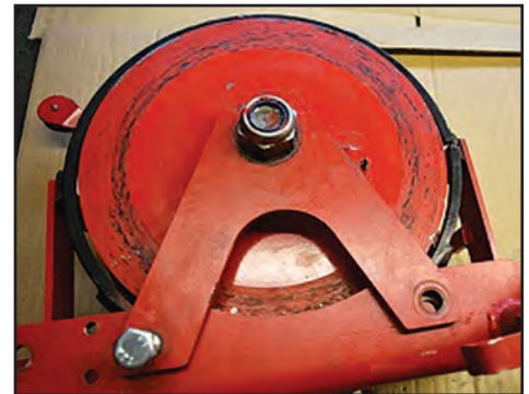
4 - Take off the connecting bolts to the drum frame unit and cable guard.
