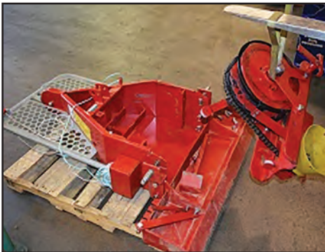
2 - Pull the drum unit from the main winch frame onto a work table.
