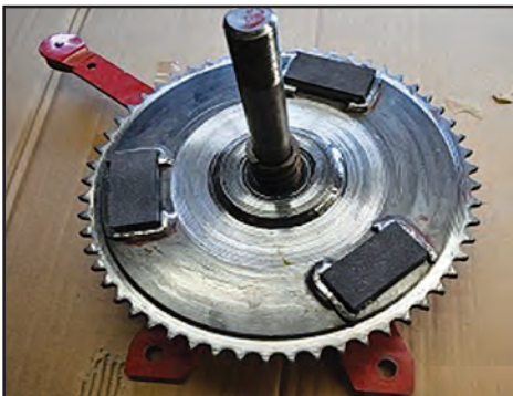
11 - Pictured are the clutch pads placed onto the clutch pad boxes.
