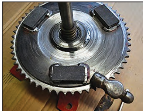
12 - Use a hammer again to "pean over" the box brackets to hold the clutch pads in place.
