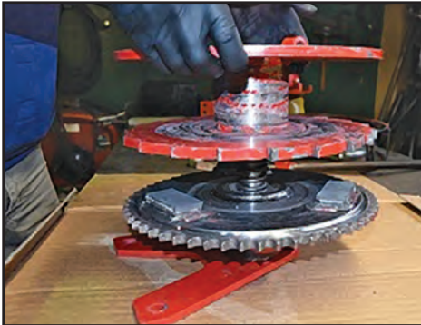
8 - Lift the drum off the main shaft and clutch assembly to get to the internal brake pads.
