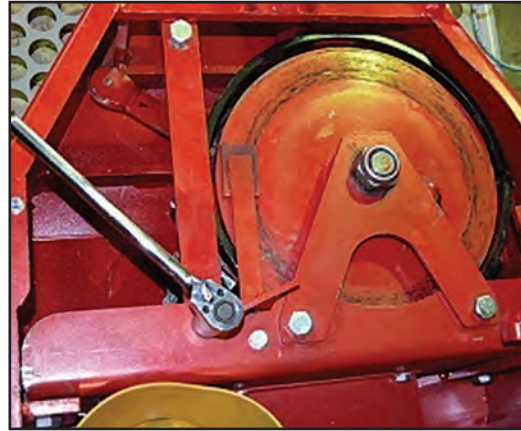
1 - Take off the 6 main drum bolts from the main winch frame unit and drum brake.
