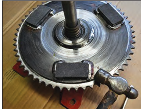
9 - To remove the old clutch pads use a hammer to "unpean" the connecting box brackets.
