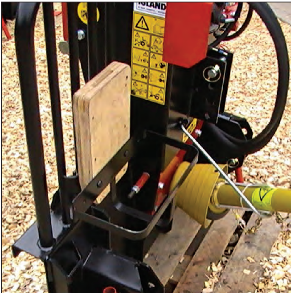
The gas can and saw brackets attach to the inside of the protective grill. Convenient and durable.
