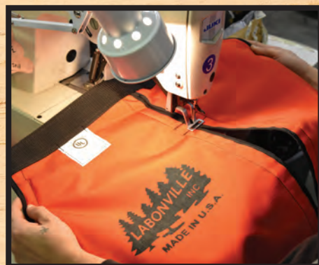
Bar tacking more critical stress points.
