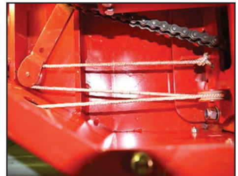
13 - This photo shows how the pulley rope system should be attached.
