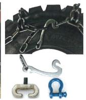
4-Use the inc. boomers and links to tighten chains.
