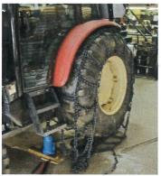
2-Once on, roll the tire and cut the excess chain.
