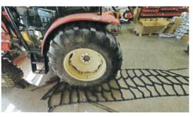
1-Lay the chains out so the studs are facing the ground and the chains are centered on the tires. If on cement as shown, jack it up not to damage the concrete. If on the ground, tie a rope to the end links, loop the rope over the tire threads and slowly roll your chains on. Be sure once on that they are centered on the tire.
