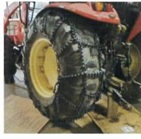
3-Start by tightening the inside chain then the outer side chains and tighten.
